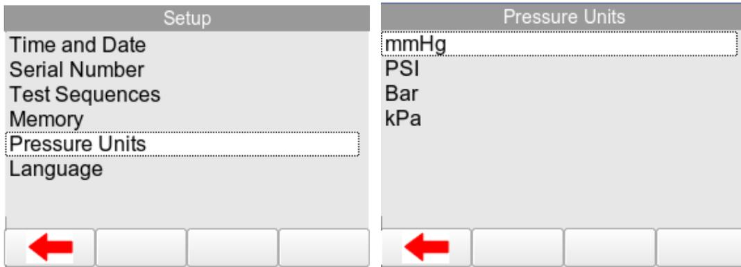
The Pressure Unit screen has a list of possible unit measurements.
