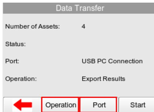
Change the data format type by pressing the OPERATION F2 button between:
