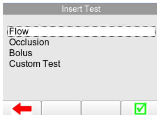
Highlighted the required test (in this example FLOW) using the rotary encoder and press to select or
