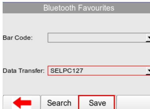
Check that the correct devices are paired for each function and press the back arrow to exit and complete the pairing;
