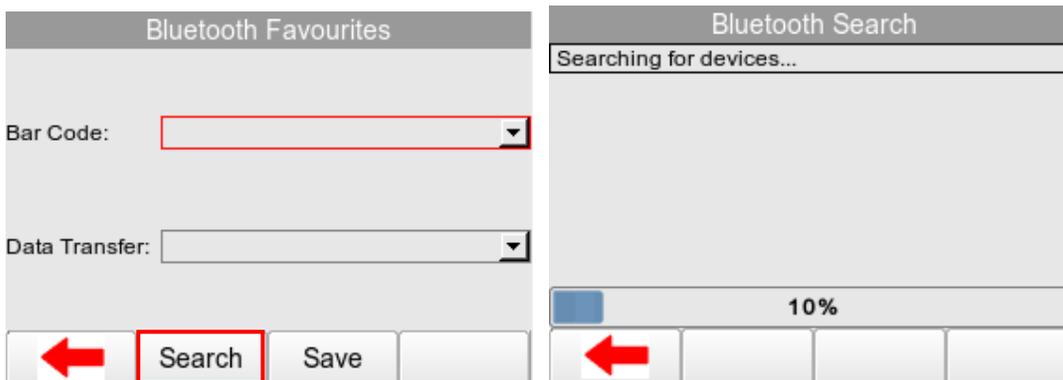
The devices found in range will be listed. Wait until the search has been completed which can take up to 15 seconds. Once the search is completed, press the back arrow key F1
