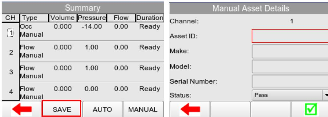
Highlight the required channel and then select SAVE F2 to save the manual test results. Parameters and asset details can then be added to the results:
