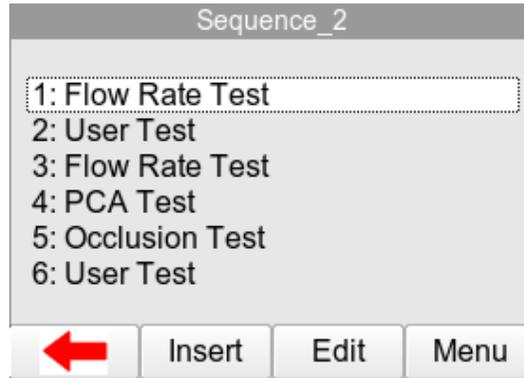
Edit individual tests by selecting the required test and press EDIT F2 on the Edit Test Sequence Menu.
