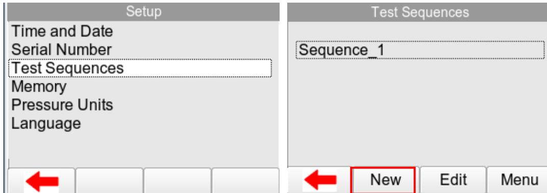
Select NEW F2 to open a new test sequence and enter a name, use the rotary encoder or USB keyboard to enter data. For the example Sequence 1 will be created.
