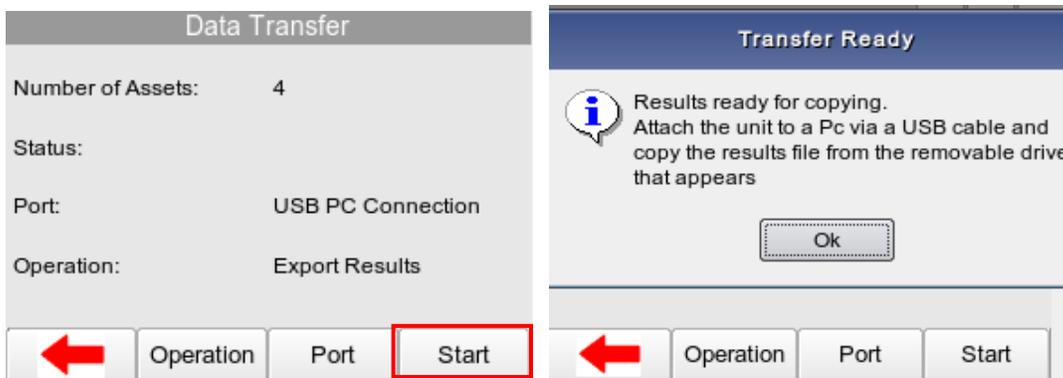
In the Transfer Ready screen connect the Rigel Multi-Flo to the PC using a USB cable.
