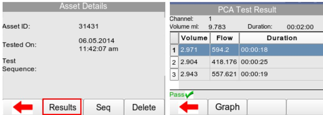
Test results can be viewed by pressing the RESULTS F2 button; test settings can be viewed by pressing TEST SEQ F3 button and the asset result can be deleted by pressing the DELETE F4 button.
