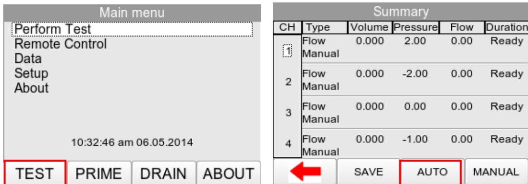
To enter the automatic mode, select TEST F1 from the Main Menu and then AUTOMODE F3 to enter the ASSET DETAILS Menu.
