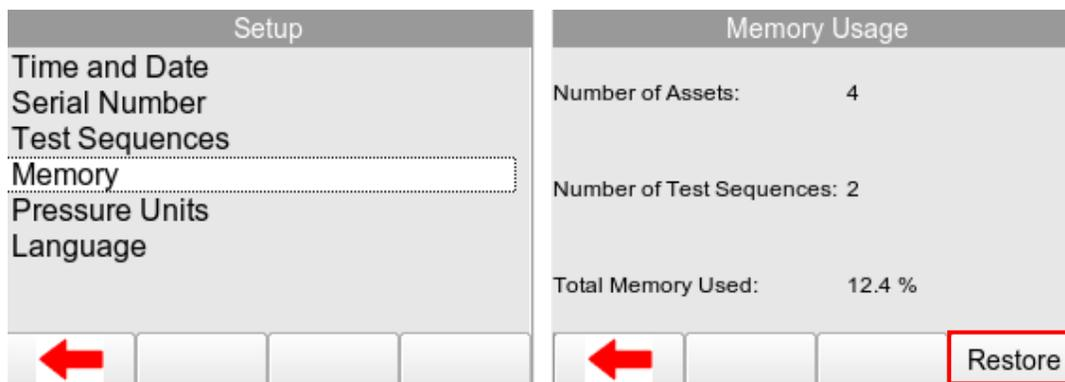
The Memory screen indicates the number of assets and test sequences stores and also the total memory used on the Multi-Flo.
