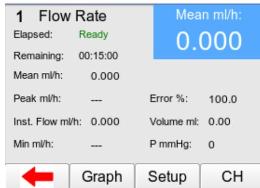
Setup your infusion device to the same settings as entered into the Multi-Flo and start the infusion. Press the green START button on the Multi-Flo to begin the test.
