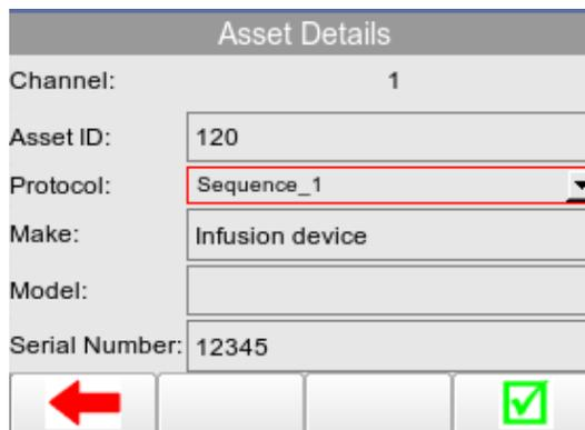
When using the barcode scanner, ensure the barcode scanner is paired with the Rigel Multi-Flo, see Chapter 6. When the barcode is ready to scan, the word “OK” will appear in the asset ID field.
