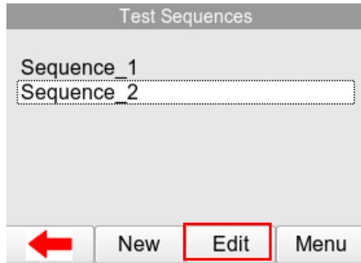
Press the EDIT F3 button to open the new test sequence for editing;
