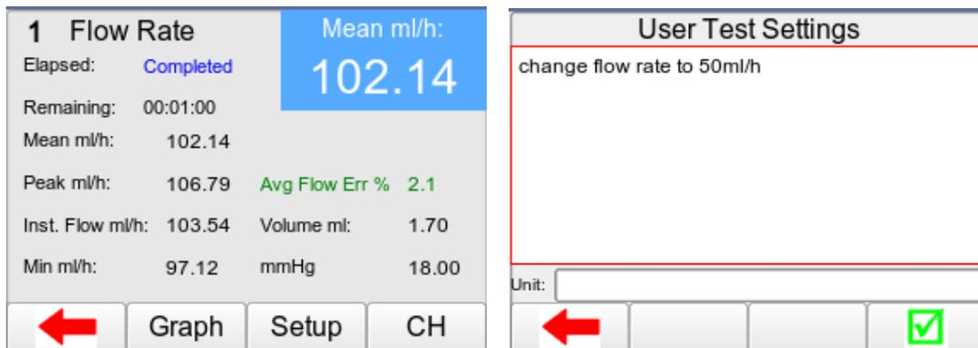
For the User test, either press **PASS** F4 or the **GREEN** button to continue, or the **RED** button to indicate that the user test could not be completed. If it is not completed the Failure menu would appear, see Chapter 3.1 for more details.
