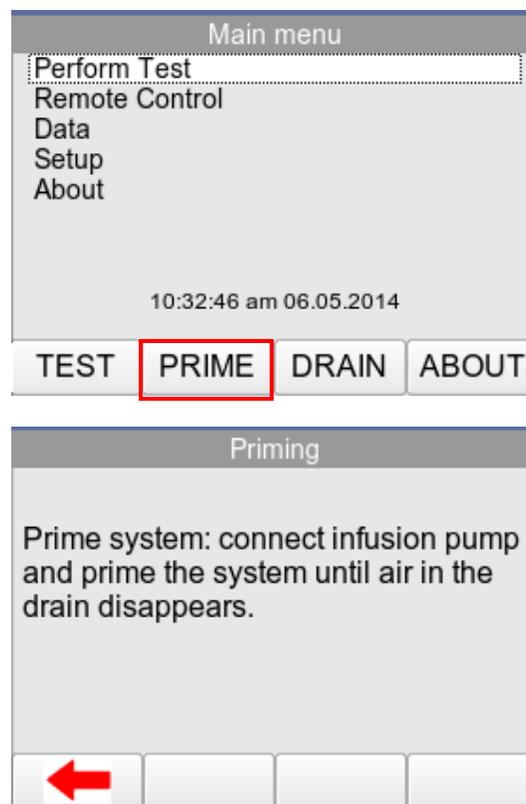
Prime the system until the drain tubing is clear of air bubbles. Press
