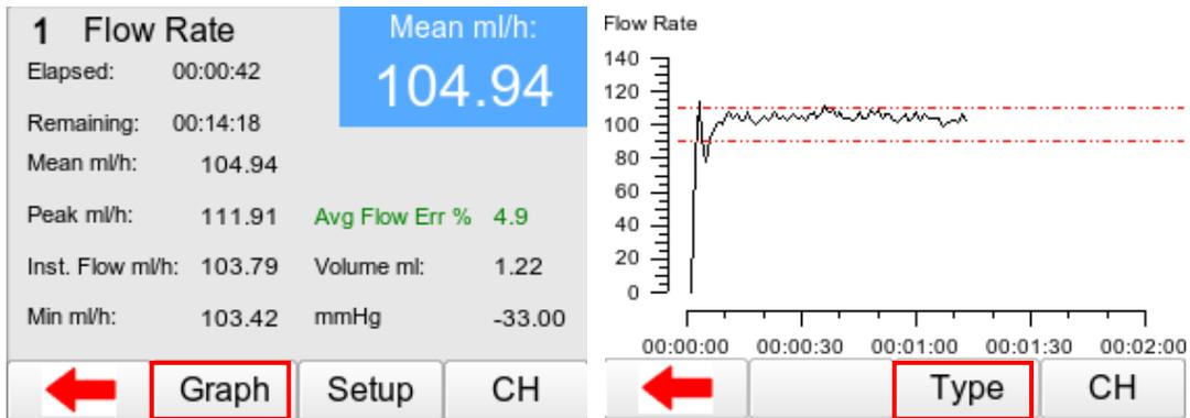
During the flow/volume test select GRAPH F2 to view the graph of the real time results. The red lines depict the set minimum and maximum limits.
