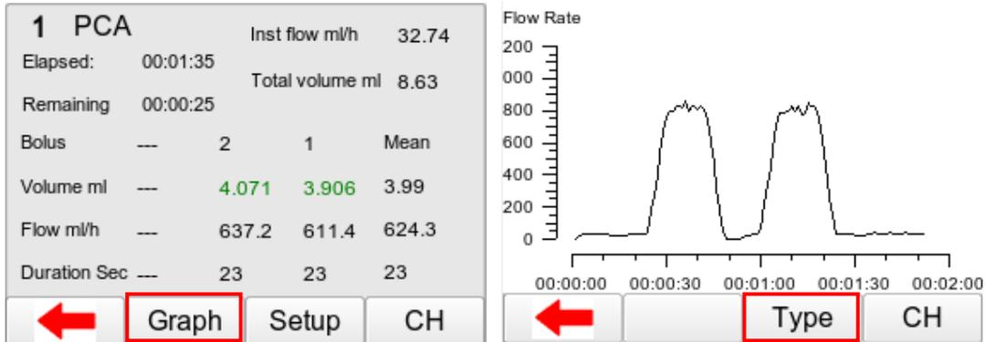
During the PCA test select GRAPH F2 to view the graph of the real time results.
