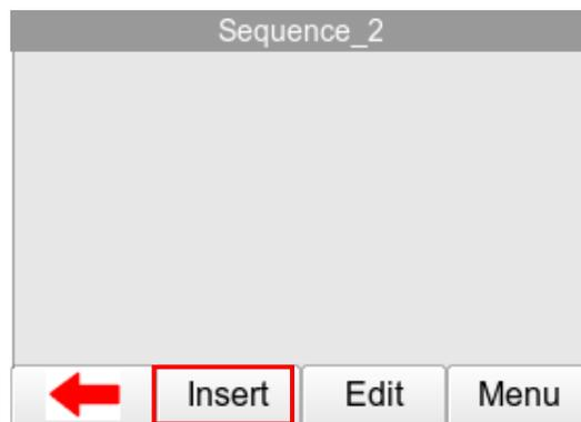
The newly created Test Name now appears in the Test Sequence menu and can be modified to include the required individual tests. Press the INSERT F2 button to open the sequence for editing and start adding individual tests to the test sequence by pressing the button.
