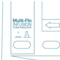
To turn the Multi-Flo ON, press the orange I/O key so it is in the in position.
