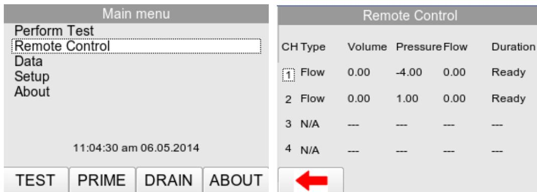
Once in the remote control menu the user will need to go onto Med-eBase software and enter the remote control manager to control the multi-flo testing.
