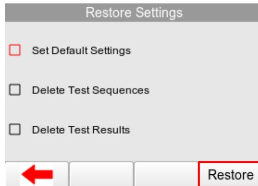
Select RESTORE F4 and a confirmation box will appear. Press the rotary encoder to select OK. Turn off the Rigel Multi-Flo to allow restore to complete.
