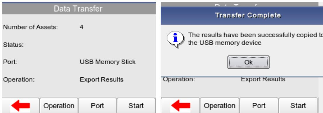
The Memory stick acts as a REMOVABLE DISC data storage device. The data file is copied from the Multi-Flo onto the drive. The files that then be stored, transferred into MedeBase and between Multi-Flo devices and PCs.
