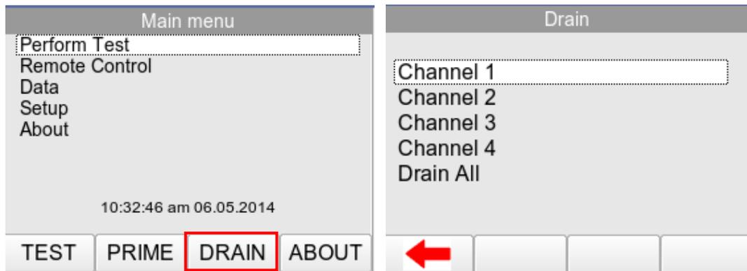
Either select the individual channel to drain or select Drain All using the rotary encoder.
