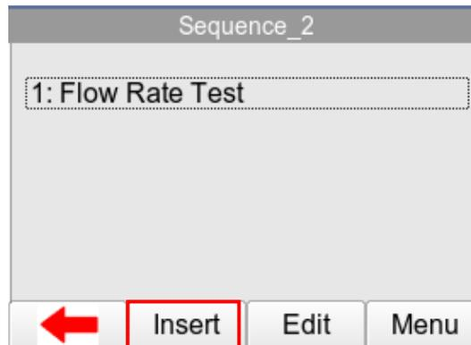
Repeat the above steps until the required test sequence is completed. Additional tests can be inserted in the test sequence by highlighting the position in the sequence and press the ADD F2 button. The test will be inserted AFTER the highlighted position.
