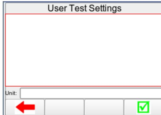
In case the user test requires data entry such as a result, the user test can also include an engineer unit such as Ohms, Watts, and Celsius etc. Confirm the entry by pressing the confirm by pressing
