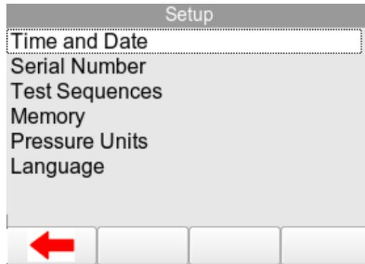
Highlight either Time / Date you wish to change using the rotary encoder and push to enter. Use the rotary encoder to increase or decrease the value then push again to confirm. Alternatively, use a USB keyboard to enter data.
