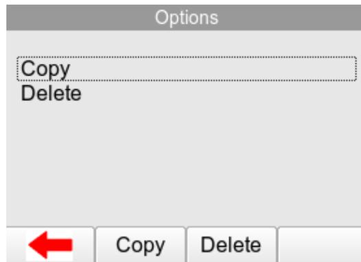
To copy, rename or delete a Test Sequence; from the Test Sequences menu, highlight the sequence required using the rotary encoder and select MENU F4.
