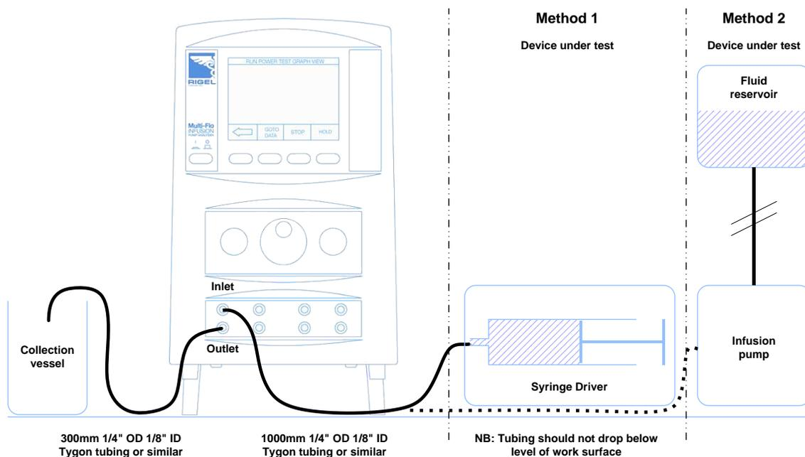
Ensure the flow direction is as per diagram above. The flow inlet is the top connection whilst the flow outlet is positioned below the inlet for each channel.
