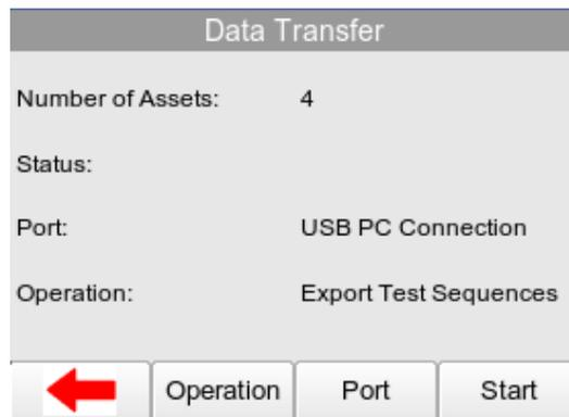
Press START F4 to connect the Multi-Flo as an external drive to the PC.
