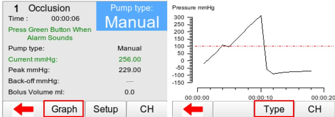
During the Occlusion test select GRAPH F2 to view the graph of pressure against time
