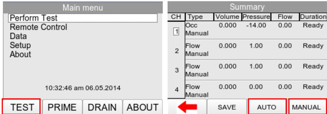
Highlight the required channel using the rotary encoder and select either MANUAL F4 to enter the Manual test setup screen or AUTO F3 to select automode to save results in the database.
