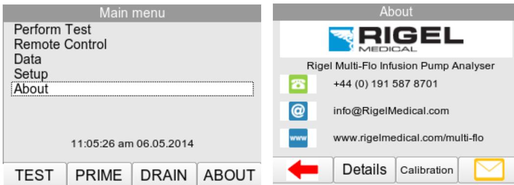
Press DETAILS F2 to view the firmware version, hardware version and serial number for the Multi-Flo unit and each individual installed channel.
